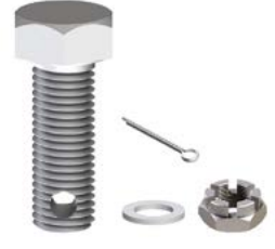
FIFTH WHEEL LOCKING BOLT MOUNTING BOLT(M16*40) BEŞİNCİ TEKER KOL SABİTLEME CİVATASI
